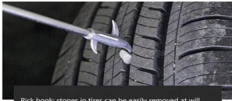
Pick hook: stones in tires can be easily removed at will
